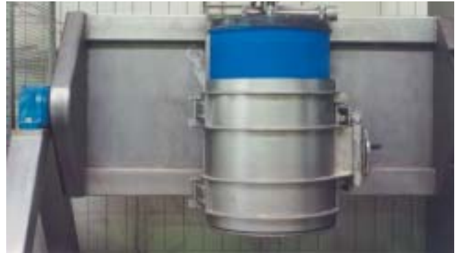
Figure 3. A reinforced clamping device ensures container stability with high-density mixes.
