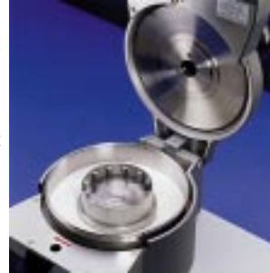
Open Ultra Centrifugal Mill showing rotor and screen. Material collects in pan.
