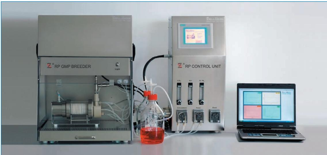
A Z<sup>®</sup> RP cultivation system comprises of Z<sup>®</sup> RP bioreactor, Z<sup>®</sup> RP GMP Breeder and Z<sup>®</sup> RP control unit. Conducted in the sterile environment of a Z<sup>®</sup> RP GMP Breeder manifold types of cell and tissue culturing processes are feasible.
