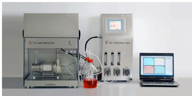
Z<sup>®</sup> RP Technology with Z<sup>®</sup> RP control unit, Z<sup>®</sup> RP GMP Breeder and Z<sup>®</sup> RP rotating bed bioreactor equipped magnetic drive and Sponceram<sup>®</sup> ceramic carrier discs
